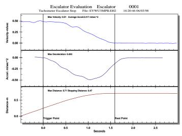
Recording & Analysis of Escalator Braking, top is the speed history, middle is deceleration, bottom is distance
