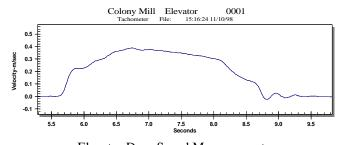
Elevator Door Speed Measurement
