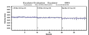
Recording & Analysis of Escalator Left Handrail, Right Handrail, and Step
