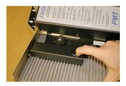
The IMD-1 would normally, already be in place, and the housing would be slid forward until the Pointer just meets the Step Edge Gauge, as shown.
