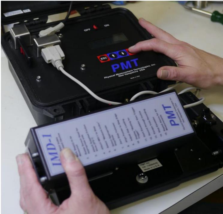
Once the Menu moves on to the next screen, the Friction Shoe Plate can be released.
