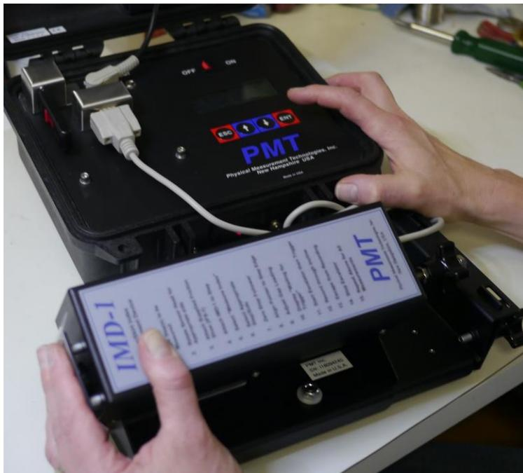
Then Press the ENT key while continuing to hold the plate fully bottomed, as shown below.
